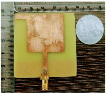
Fig. 14 Fabricated design of proposed antenna
