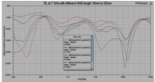
Fig. 5 S<sub>11</sub> of Patch antenna with different ground plane effect Lg.
