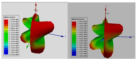
Fig. 8 Directivity of patch antenna at 7 GHz & 3D Polar Gain in db at 7GHz
