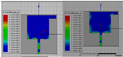
Fig. 11 E Field at 7GHz & H Field at 7GHz
