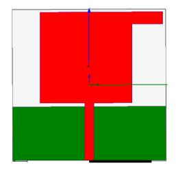
Fig. 2 Geometry of rectangular patch
